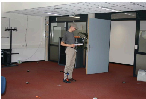
(c) Snapshot of data collection performed by the user within the lab. Deployed ultrasound nodes are shown as black boxes on the floor.
