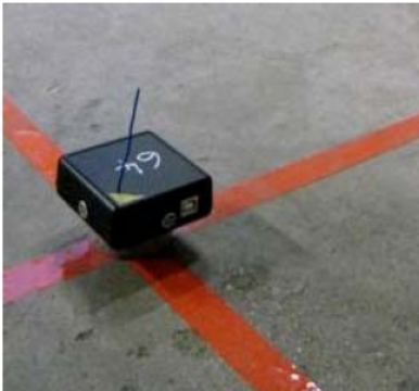
(a) Ultrasound node used for deployment as landmarks.
