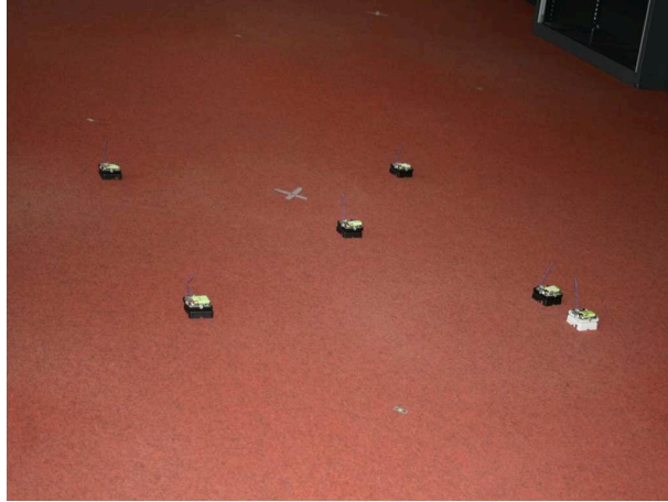
Figure 6.4: Placement of ultrasound nodes used for raw measurement characterisation. Sender node placed at successive points for a few minutes, while the remaining nodes were made to listen for the ultrasonic transmissions from the sender.
