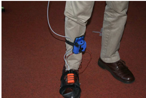
(b) Ultrasound node (blue) and Xsens inertial unit (orange) firmly attached to user's foot
